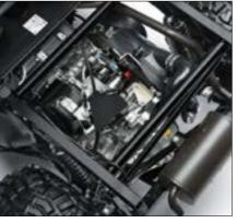
ENGINE The 401 cc, four-stroke, OHV, air-cooled engine is compact, light, durable and delivers its power reliably and economically with a restricted top speed of 40km/h (25mph).
