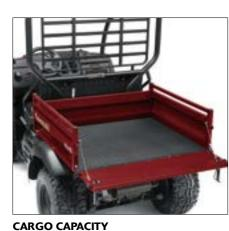
The easy-to-load tilting cargo bed can carry up to 181 kg of tools and materials while and additional 500 kg can be towed behind the ever-eager MULE.
