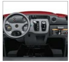
DASHBOARD Drawing on the design of the PRO Series console, the dashboard puts all controls within easy reach and sight of the operator. Thick-grip steering wheel aids comfort.
