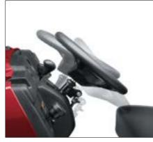
TILT STEERING The PRO Series style thickly padded steering wheel can be tilted through 29° to suit operator preference and facilitate a quick and easy entrance exit, making getting in and out of the MULE easier.
