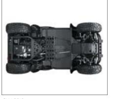
CHASSIS A tubular steel chassis provides the best balance of rigidity, strength and ride comfort. Independent front suspension and rack-andpinion steering aid traction and handling.
