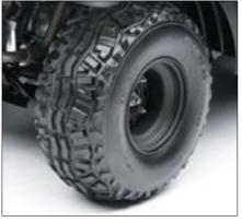
**BIG WHEEL 4X4** The MULE SX 4x4 has large 24" off-road tyres making it even easier to tackle rough terrain. Hi-Lo dual range auto transmission with rear diff lock enhance traction.
